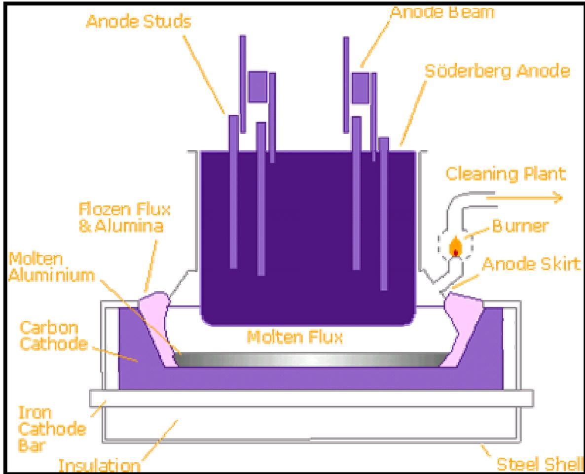
**The Anode:** As we have seen, the carbon anodes used in the Hall-Héroult process are consumed during electrolysis. Two designs exist for these anodes; "Söderberg" and "Pre-Bake". Pre-Bake anodes are made separately, using coke particles bonded with pitch and baked in an oven. Pre-bake anodes are consumed and must then be changed. Söderberg anodes on the other hand are baked by the heat from the electrolytic cell, they do not need changing but are "continuously consumed".
